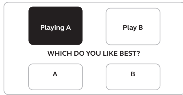
Figure 2. The interface for the preference test in the second and third experiments based on paired comparisons a provided by the web-based listening test tool SenselabOnline®.
