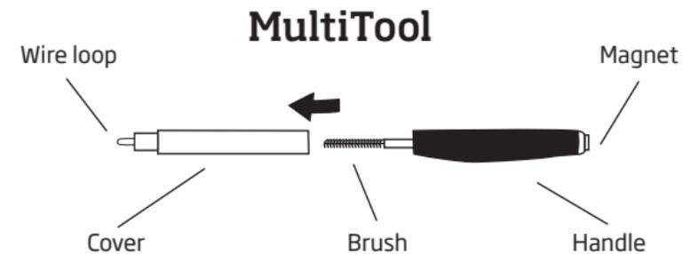
The MultiTool contains a brush and a wire loop for the special purpose of cleaning wax from the ear mold. Use the cloth to wipe clean the surface of the instrument.
