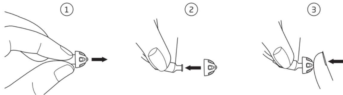
Under the dome you will notice a white wax filter attached to the end of the speaker. This is a wax filter that will keep debris from damaging the speaker. If this filter becomes clogged, contact your Hearing Care Professional for service and replacement of the filter.
