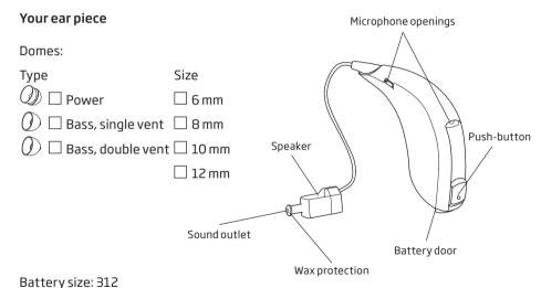
Open the battery door fully to allow air to circulate whenever you are not using your hearing instrument, particularly overnight.
