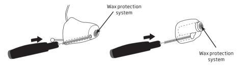
Replace the brush when necessary. Just pull it out of the tool and insert a new fresh brush. Press the new one firmly into the handle. Brushes can be purchased from your Hearing Care Professional
