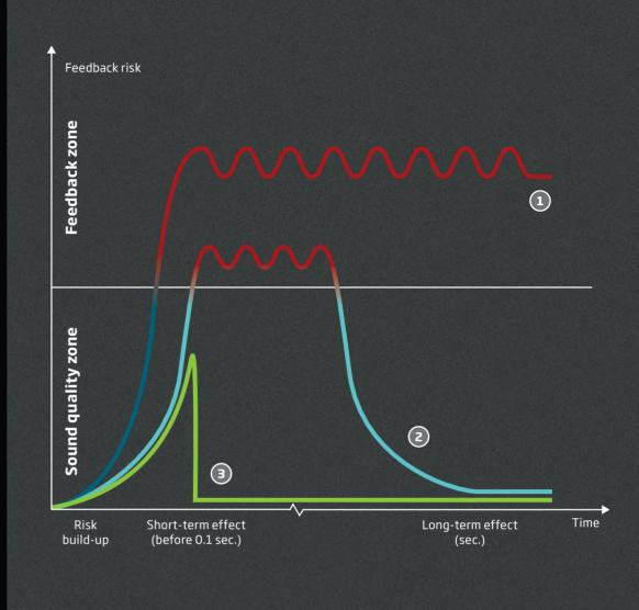
$(\mathbf{z})$ Hearing aid with conventional technology Traditional anti-feedback with slow detectors: With this reactive technology, feedback rises and becomes audible. Utilizing gain reduction and other measures, the hearing aid slowly returns to stability. Audibility, sound quality and speech understanding are compromised.
