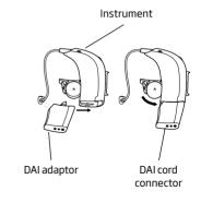
If you would like to turn off the hearing instrument microphone input and listen to the DAI alone, you can advance to the next program by using the program switch button.
