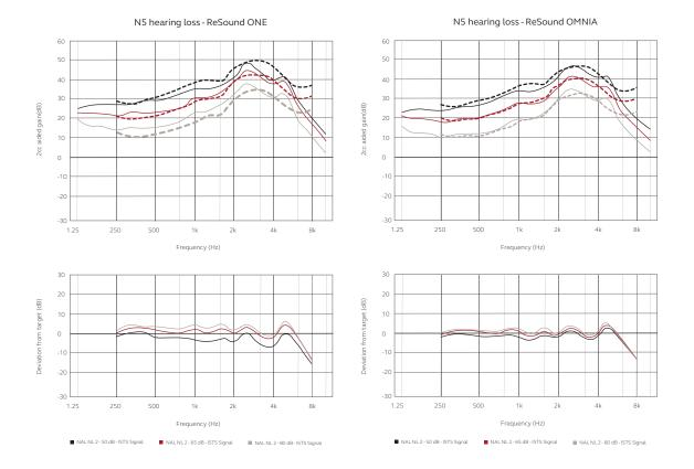
Figure 3: Comparison of 2cc coupler measurements of ReSound ONE (left panel) and ReSound OMNIA (right panel) hearing aids fit to the N5 audiogram using NAL-NL2. Dashed lines are target curves and solid lines are measurements.
