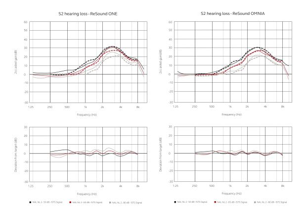
Figure 2: Comparison of 2cc coupler measurements of ReSound ONE (left panel) and ReSound OMNIA (right panel) hearing aids fit to the S2 audiogram using NAL-NL2. Dashed lines are target curves and solid lines are measurements.
