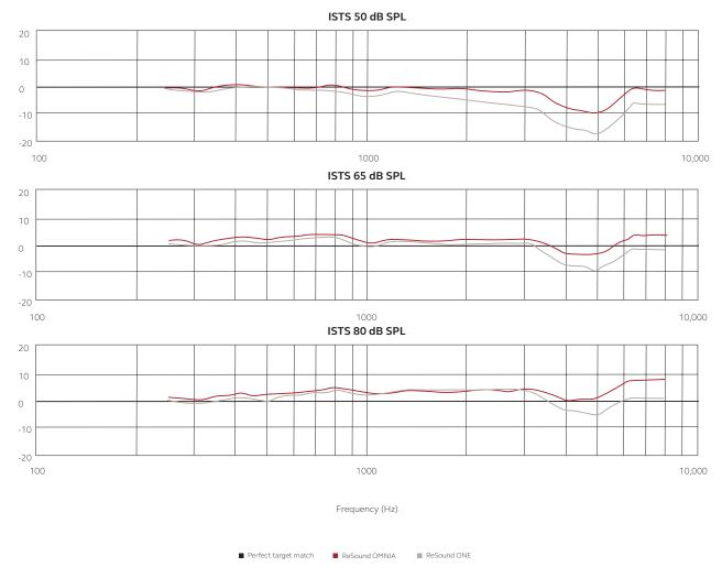
Figure 4. Deviation of mean REIG from NAL-NL2 REIG speech targets for three input levels of the ISTS signal. The solid line at 0 dB is an ideal target match, the red line is ReSound OMNIA, and the grey line is ReSound ONE.
