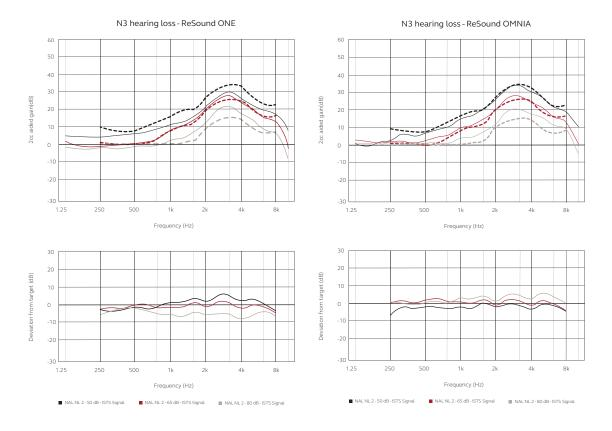
Figure 1: Comparison of 2cc coupler measurements of ReSound ONE (left panel) and ReSound OMNIA (right panel) hearing aids fit to the N3 audiogram using NAL-NL2. Dashed lines are target curves and solid lines are measurements.
