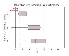
Figure 3. Maximum absolute deviation of insertion gains for different insertion qualities (score of 8, 6, 3 compared to an "ideal" score of 10). In most cases the deviation is greater than 5 dB.
