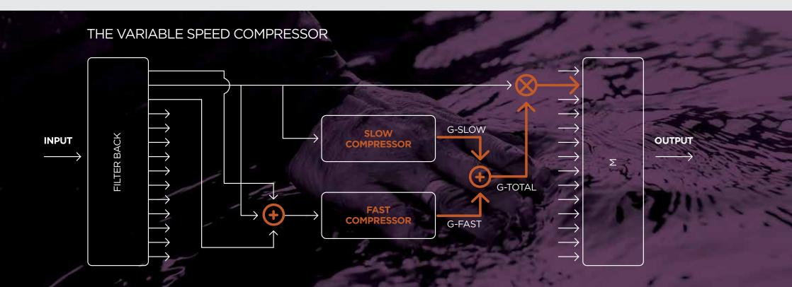
The Variable Speed Compressor comprises two separate compressors: a primary, slow-acting compressor and a fast-acting compressor working in parallel. This enables us to preserve the temporal waveform as well as the audibility cues of the system.
