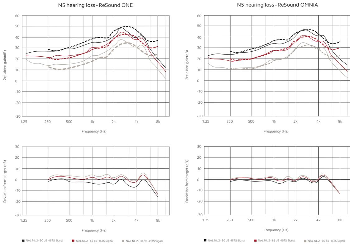
Figure 3: Comparison of 2cc coupler measurements of ReSound ONE (left panel) and ReSound OMNIA (right panel) hearing aids fit to the N5 audiogram using NAL-NL2. Dashed lines are target curves and solid lines are measurements.
