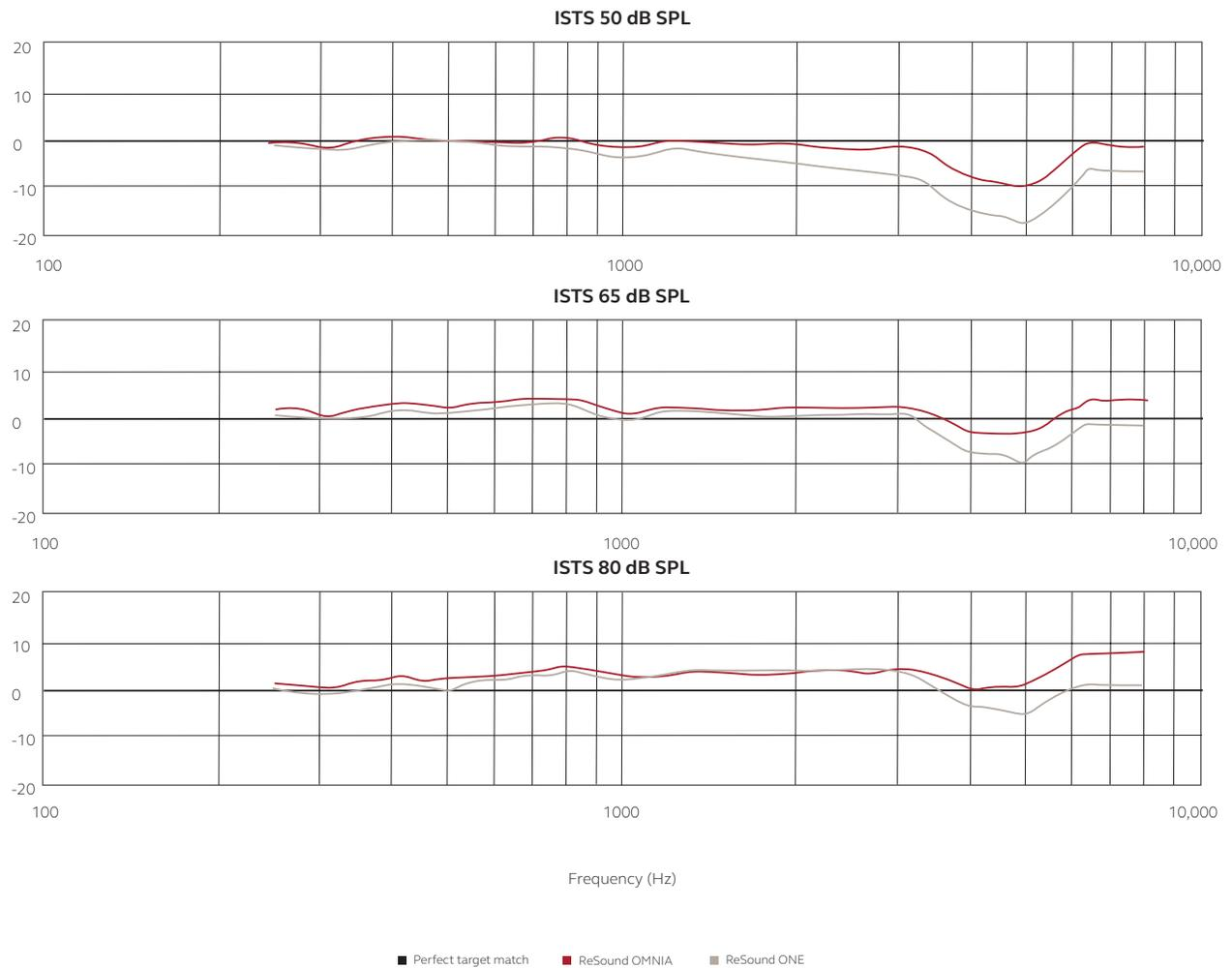
Figure 4. Deviation of mean REIG from NAL-NL2 REIG speech targets for three input levels of the ISTS signal. The solid line at 0 dB is an ideal target match, the red line is ReSound OMNIA, and the grey line is ReSound ONE.
